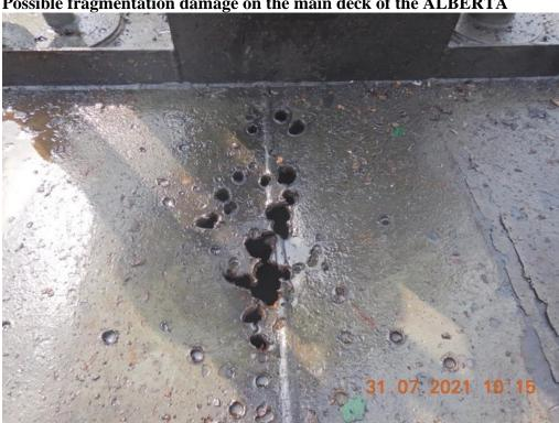
Figure 14.1 Possible fragmentation damage on the main deck of the ALBERTA
